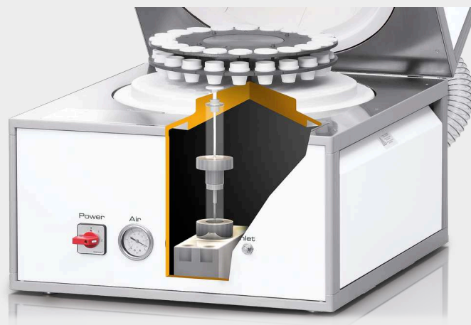
Encapsulated weighing cell
