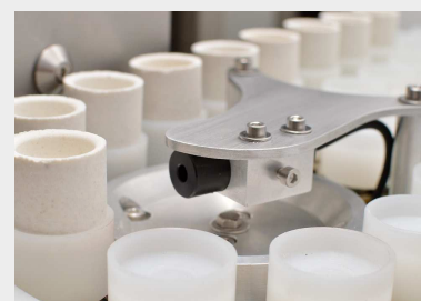
Autoloader with acid-resistant plastic crucible holders
