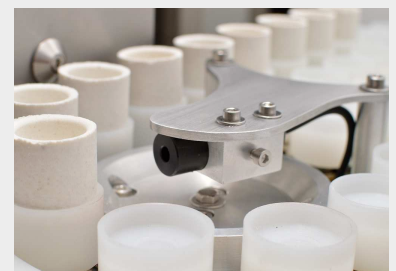
Autoloader with acid-resistant plastic crucible holders
