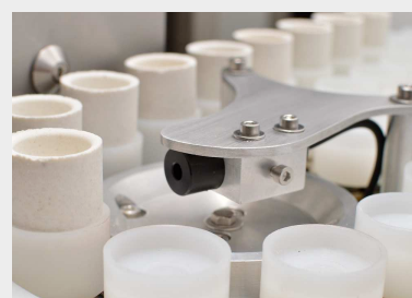
Autoloader with acid-resistant plastic crucible holders
