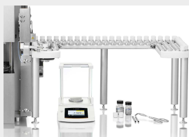
Autoloader with 130 crucible positions
